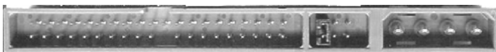
Fig. 4.13 Parallel ATA disk drive sockets and jumpers (photograph: Tony Sammes and Brian Jenkinson).
